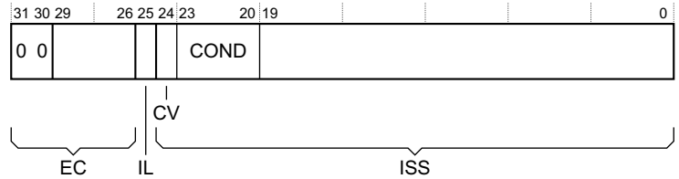
Figure G4-19 HSR format when the ISS includes CV and COND fields
